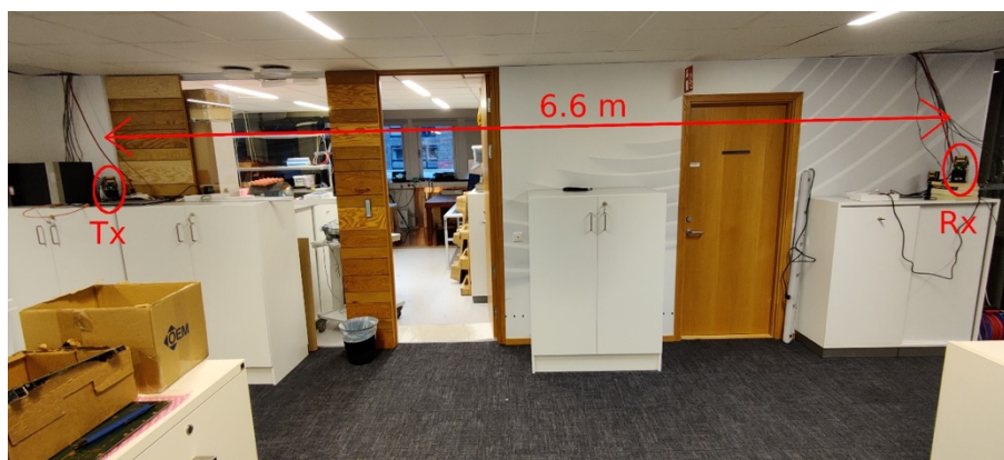
Figure 5-18 Measurement setup with Tx radio to the left and Rx radio to the right, separated by 6.6 m. Both radios are oriented facing 45° from each other out from the wall.
