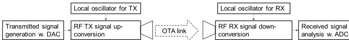
Figure 3-4: High level block diagram of extreme data speed proof-of-concept demonstrator arrangement.
