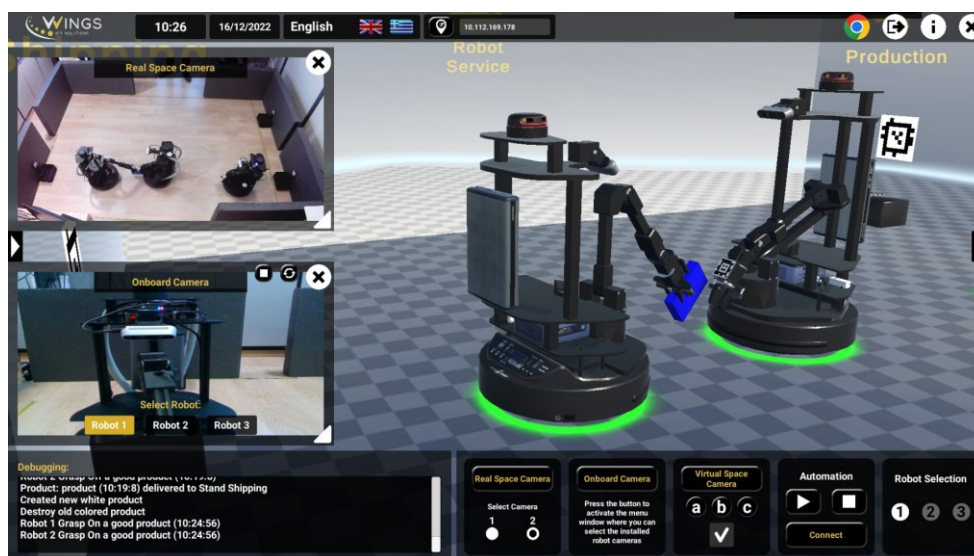
Figure 6-7: Digital twin interface showing the moment a product is exchanged between two robots.
