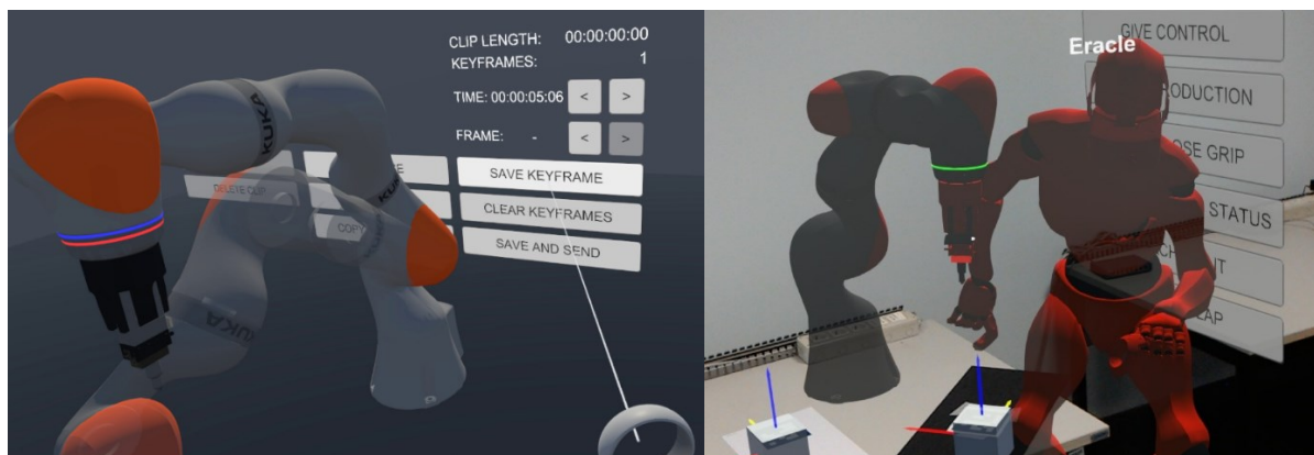
Figure 5-4: RU (expert) in the act of creating a program clip to be used to train the LU (left), and RU's avatar as seen by the LU during the same activity (right).
