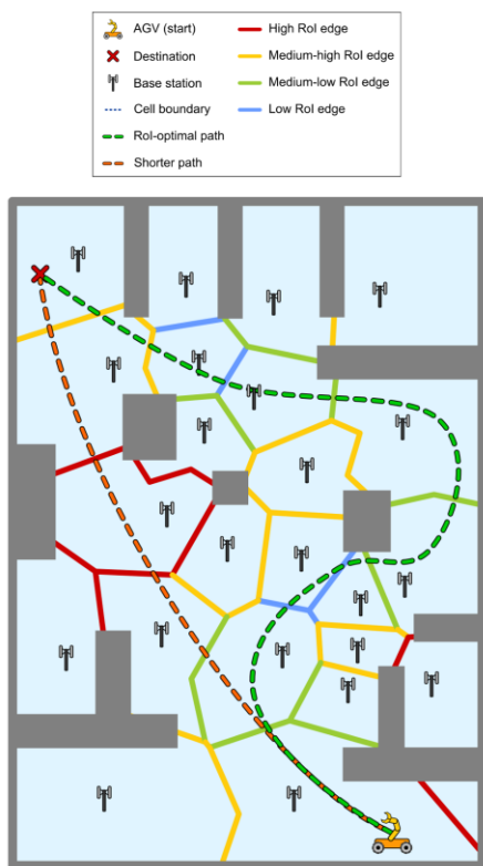
Figure 3-12: Depiction of a RoI-optimal path calculated by the vehicle from the RoI values at the cell edges, which minimizes the crossing over cell edges with high interference risk.
