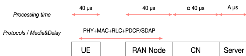
Figure 6-2: Latency components of single RAN with co-located CN.
